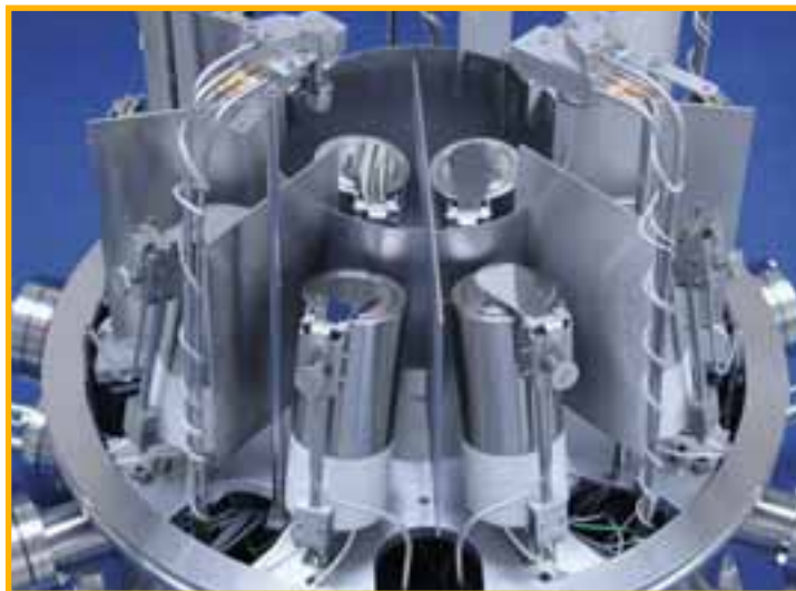
Custom 12 LTE organic source array with integral flip shutters
